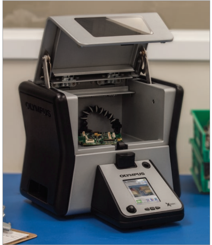
Secure small objects in the sample-holder to orient on the analysis window.
