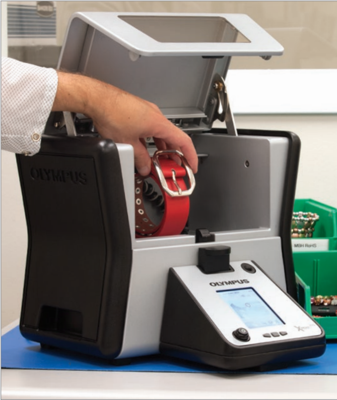
The Xpert is easy-to-use. Place large objects directly on the analysis window.
