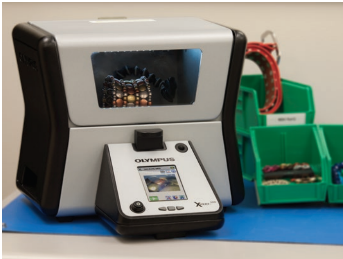
Integrated CMOS camera records sample images to memory.
