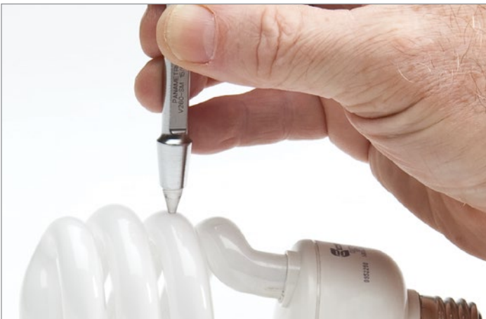
Measure thin glass with a V260-SM Sonopen® transducer.
