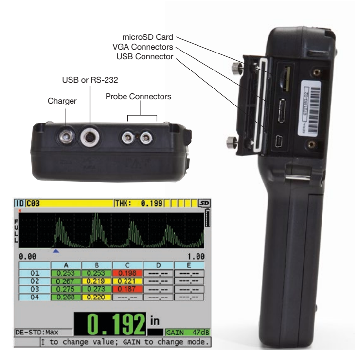
Onboard DB Grid View with three programmable colors
