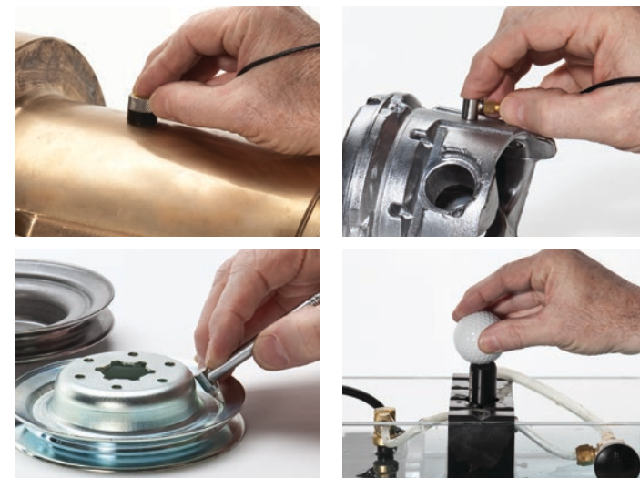
Ultrasonic thickness measurements are accurate, reliable, and repeatable. Instant readings can be achieved from one side of a material, making it unnecessary to cut up or destroy the part.
